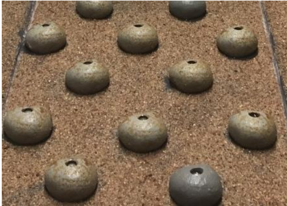
Figure 1. 95-mm roughness elements were spaced one diameter apart in a chevron pattern. The surface texture treatment shown in this image is the sand (1 – 2 mm diameter) treatment.
